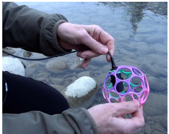
CUSTOM HYDROPHONE BY AMBEINT RECORDING GMBH MUNICH
